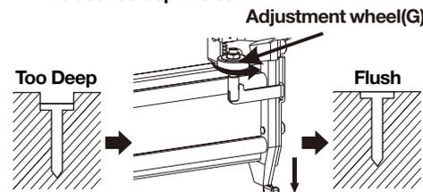
Turn the adjustment knob counter clockwise
