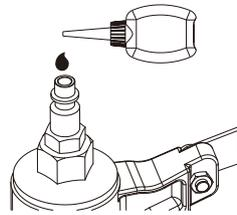
3. After adding oil, connect the tool to the air source, run tool briefly. Wipe off any excess oil from the cap exhaust.
