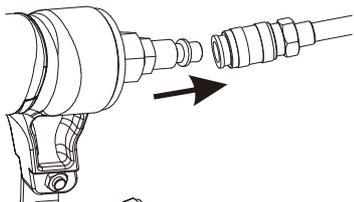
2. Turn the tool so the air inlet is facing up. Place 2 - 3 drops of pneumatic fastening tool oil into air inlet. Do not use detergent oils, oil additives, or other air-tool oils as these lubricants will cause accelerated wear to the seals and bumpers in the tool, resulting in poor tool performance and frequent tool maintenance.
